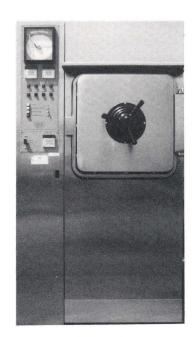
A chamber pressure gauge is provided and is visible to the operator. A cycle recorder is mounted in the control panel and is visible to the operator. The cycle recorder is the dual pen type to record pressure and temperature. The pens record in contrasting colors for easy distinction between pressure and temperature tracings. An audible alarm signals the cycle completion. Cycle mode indicator lamps provide at a glance cycle progress. Timers automatically re-set.
